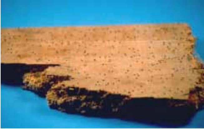
Figure 4. Larvae of the Queensland pine beetle can reduce susceptible timber to fine gritty cigar-shaped pellets.
